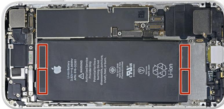
**i** The iPhone's battery is secured by four pieces of stretch-release adhesive—two at the top, and two at the bottom.
